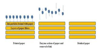
Fig. 1. Diagrammatic representation of enzymatic deinking of paper.
